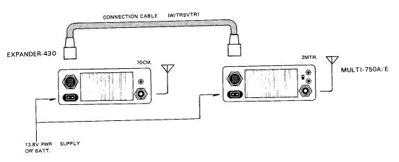
The special connecting cable should be plugged into the rear of the MULTI-750A/E and EXPANDER-430 transverter unit.
